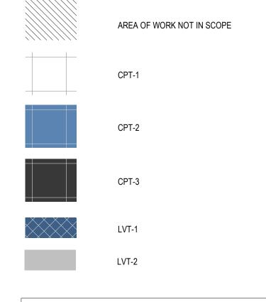
NOTE: ORIENTATION OF HATCH DOES NOT INDICATE DIRECTION OF CARPET/LVT FLOORING
